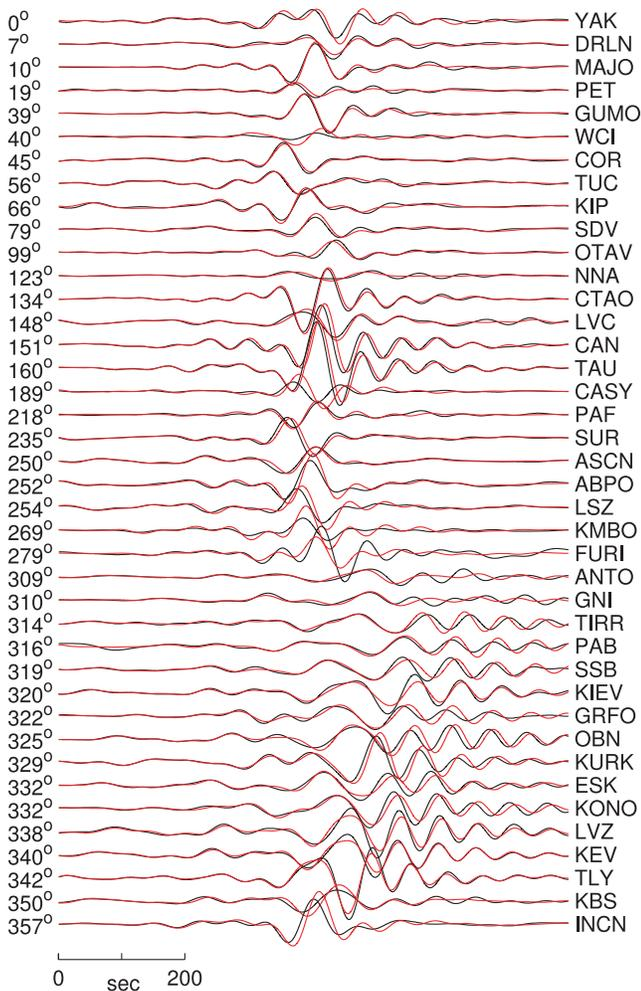
**Figure 8.** Transverse component record section comparing data (black) and SEM synthetics (red) for the 2007 August 17,  $M_w = 6.4$ , Banda Sea earthquake, which occurred at a depth of 21 km. The records are aligned on the Love wave (using a  $4.4 \text{ km s}^{-1}$  phase speed), plotted as a function of source azimuth, and bandpass filtered between 60 and 200 s. Source azimuth is plotted to the left of each set of traces, and FDSN station identification codes are plotted to the right.
