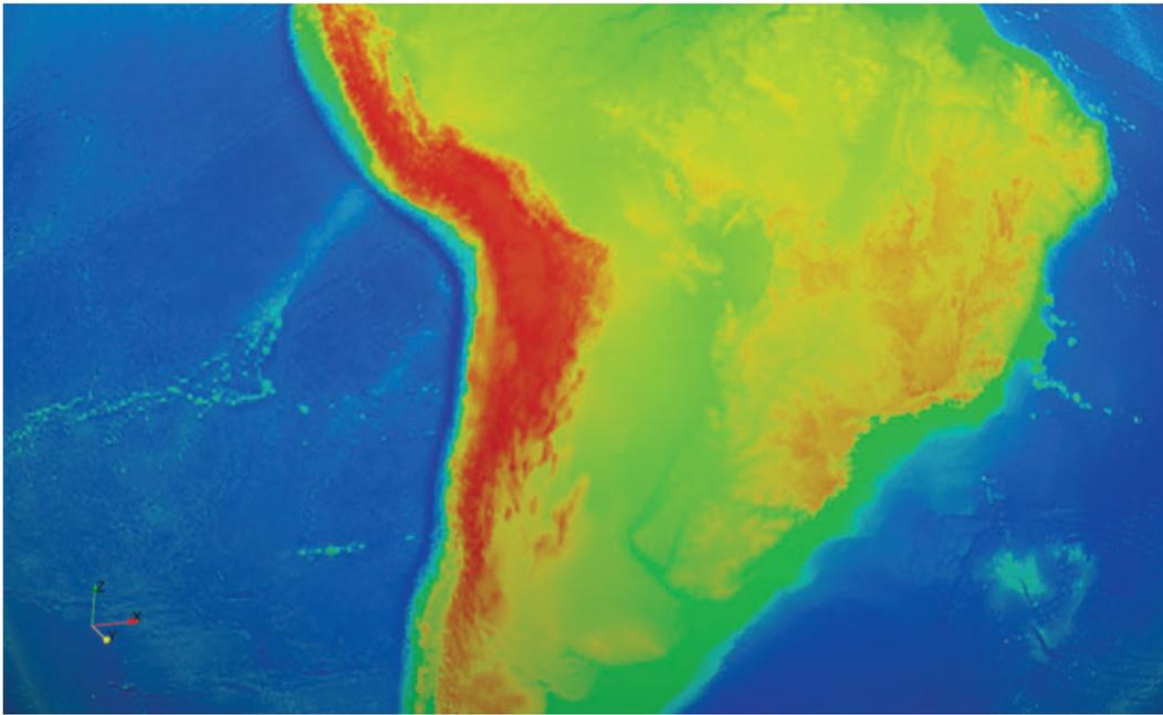
**Figure 5.** Each spectral element at the Earth's surface has  $3 \times 3 = 9$  finite-element anchors in its top face, and these are used to capture topography and bathymetry. Shown are surface elevations in South America as captured by the spectral-element mesh used in the near real-time 3-D SEM simulations.
