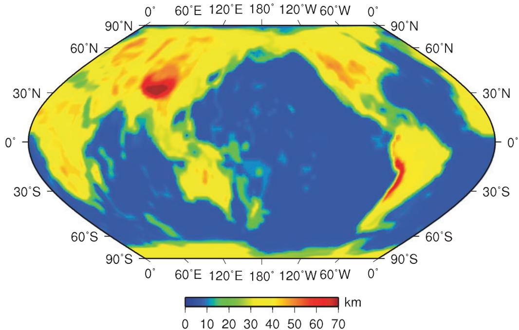
**Figure 2.** Map of crustal thickness obtained by smoothing  $2^\circ \times 2^\circ$  block model Crust2.0 (Bassin *et al.* 2000) with a one-degree Gaussian cap. The Moho is honored in the spectral-element mesh as a first-order discontinuity if the crustal thickness is less than 15 km (one spectral element) or greater than 35 km (two spectral elements), as shown in Fig. 3.
